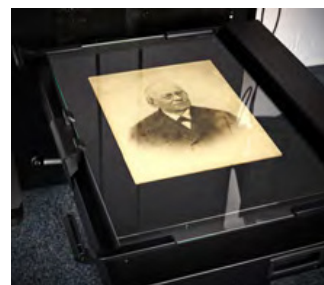
Photo table with glass plate and soft pad for very careful handling
