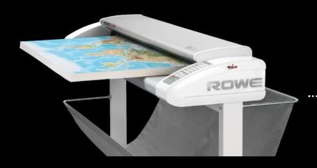
Automatic height adjustment up to 30mm /1.18". The ROWE Scan 850i scans even the thickest originals- up to 30mm (1.18")-a user wish which was often expressed. The electrically driven ROWE HEIGHT ADJUSTMENT works automatically at the simple push of a key: sensors determine the exact thickness of the original, the top part of the scanner positions itself automatically at the correct height and the ROWE SAFE DRIVE guarantee the safe transport of the original.
